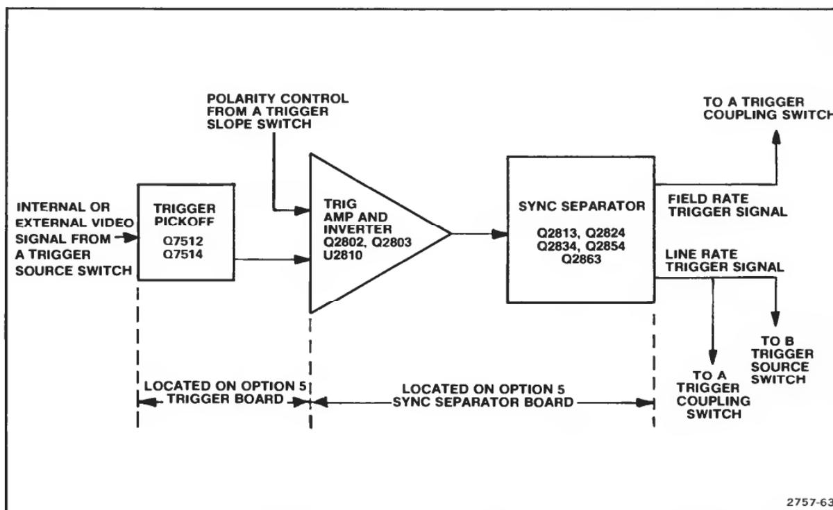
Figure 6-3. Option 05 simplified block diagram.
