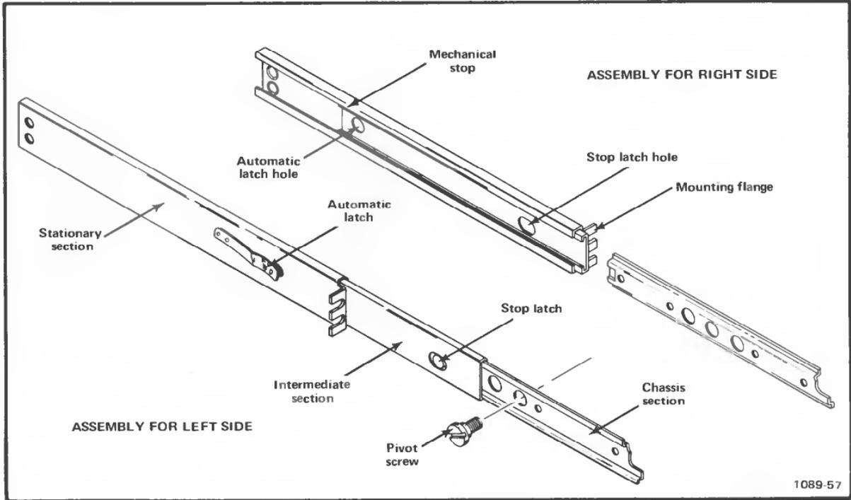
Figure 2-10. Slide-out track assemblies.
