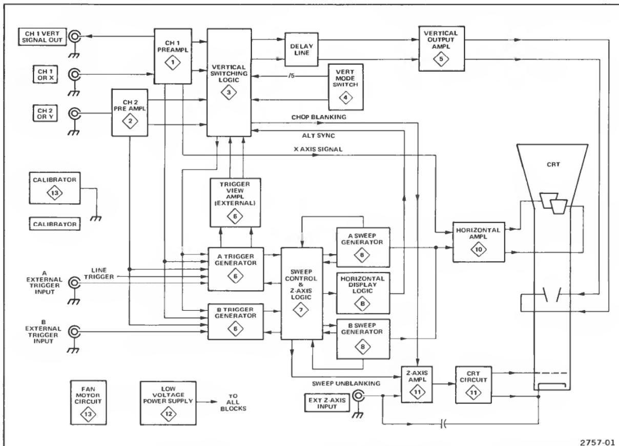
Figure 3-1. Basic block diagram of the 465B Oscilloscope.
