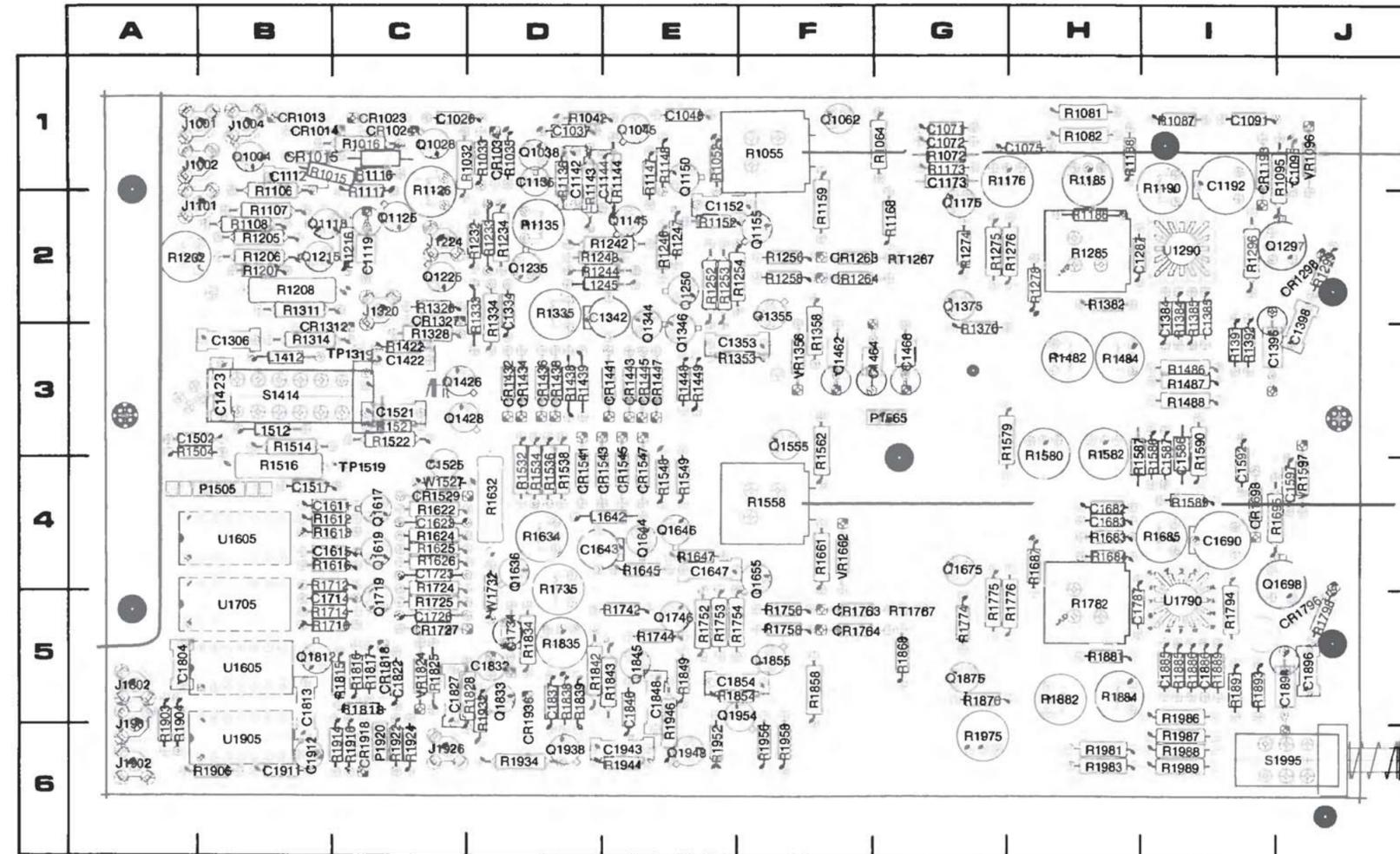
Figure 8-3. A1 Vertical Preamplifier circuit board.
