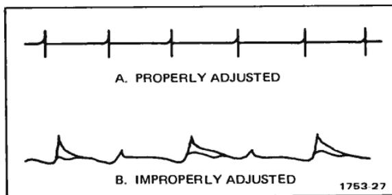
Figure 6-12. Option 07 Inverter balance.
