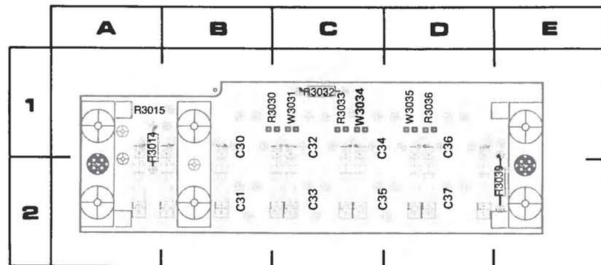
Figure 8-2. A3-Attenuator circuit board.
