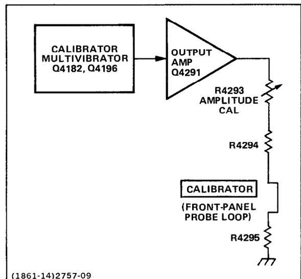
Figure 3-12. Detailed block diagram of the Calibrator circuit.
