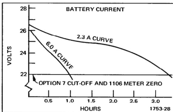
Figure 6-11. Typical battery pack discharge curves.
