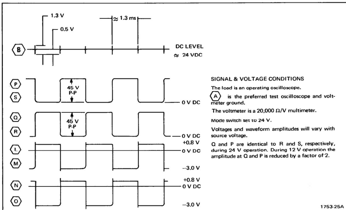
Figure 6-14. Option 07 DC Inverter idealized waveforms.
