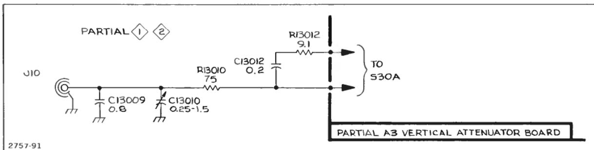
Figure 6-5. Option 05 465B Vertical Input changes.
