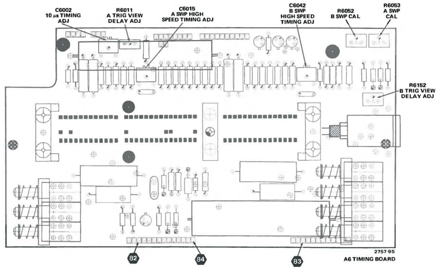
Figure 8-14. Timing circuit board adjustment locations.
