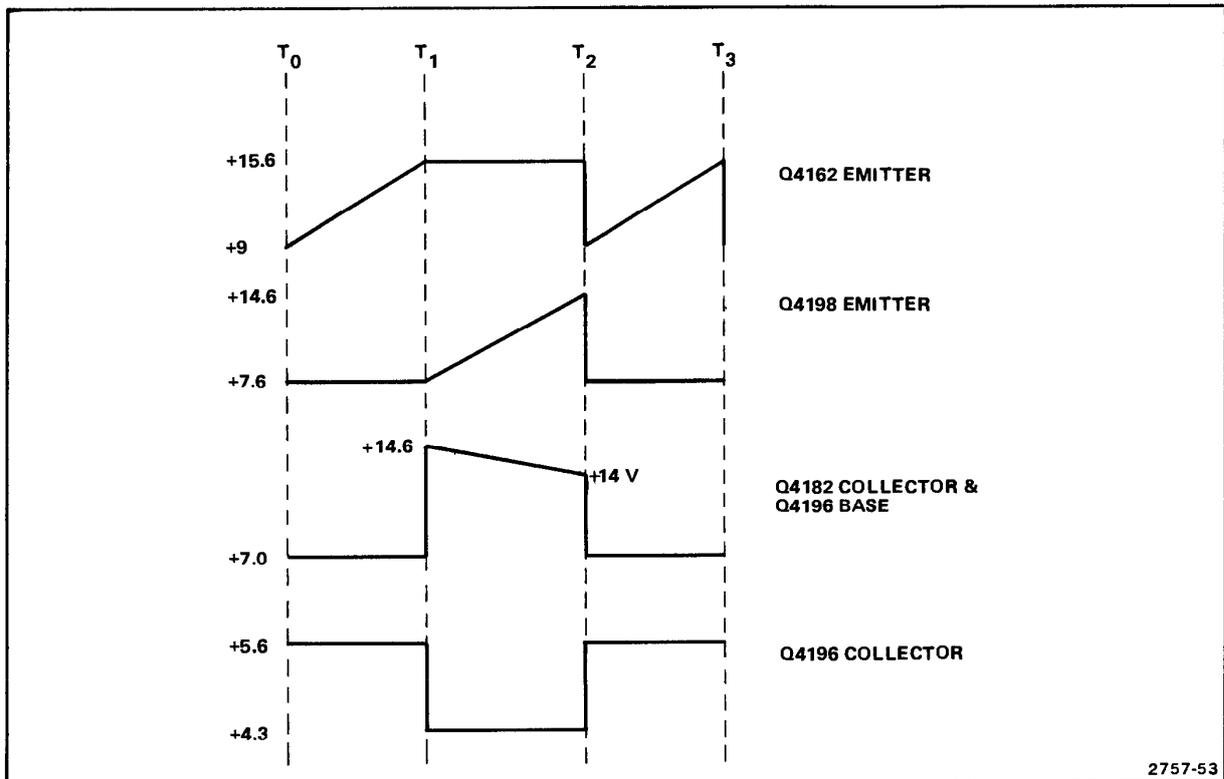
Figure 3-13. Calibrator circuit waveform diagram.
