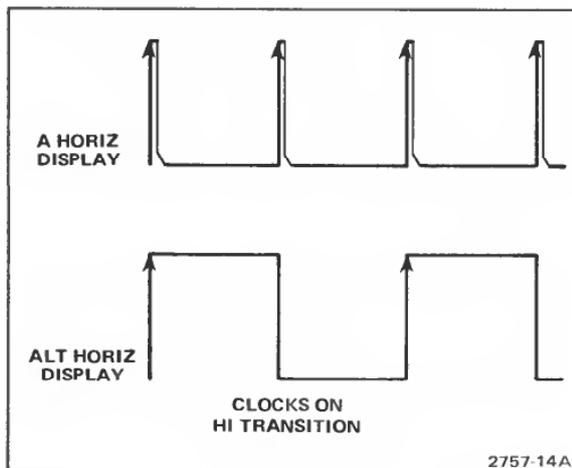
Figure 3-5. Vertical Alt Sync Pulse at U1705 pin 9.
